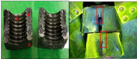
Fig. 2 Crack of wedge nut
