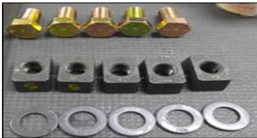
Fig. 7 The specimens of screw torque test
