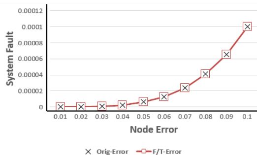
Figure 14. Comparison of error in the original and F/T Full replication algorithm ( S=4 )
