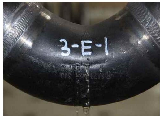
Fig. 4 Fatigue crack on specimen
