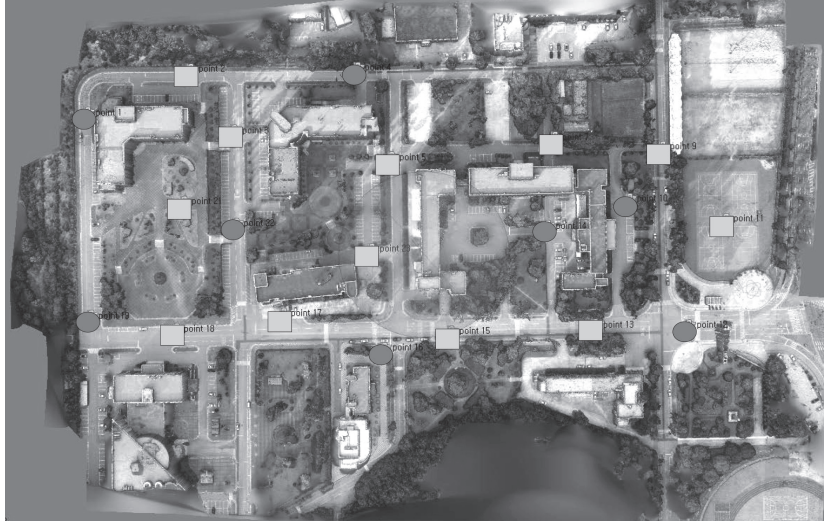
Fig. 2. Test area and distribution of control points (GCPs: red circles, check points: orange rectangles)
