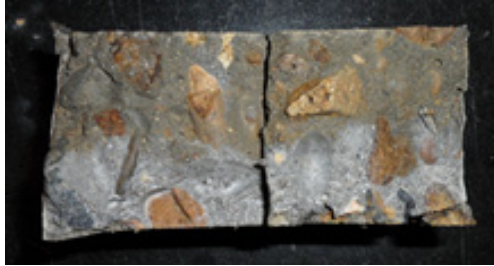
Cold joint - 60% loading level
