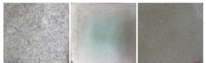
(a) Granite (b) Normal concrete (c) UHPC
