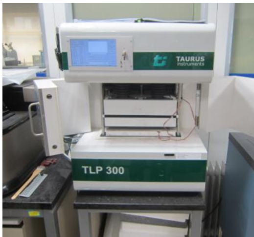
Fig. 11 Instrumentation for measurement of thermal conductivity
