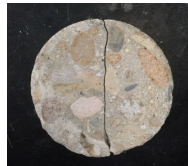
Fig. 6 Photo for disk concrete(Tensile)
