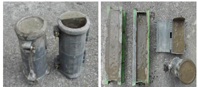
Fig. 2 Photos for concrete containing cold joint
