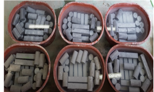
(c) Specimens under curing
