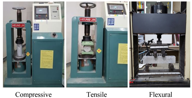
Fig. 3 Photos for compressive, tensile, and flexural strength test
