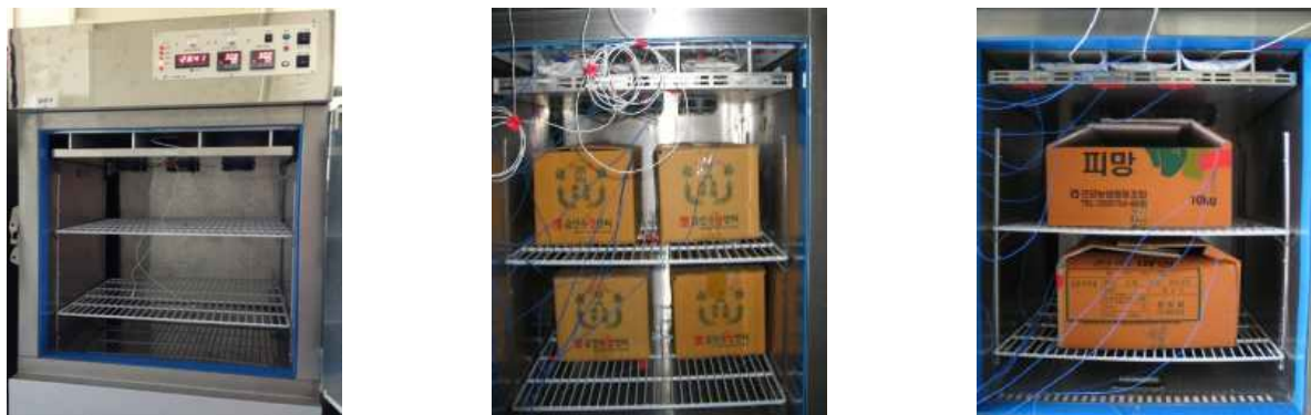
Fig. 1. Transportable thermoelectric cooling system.
