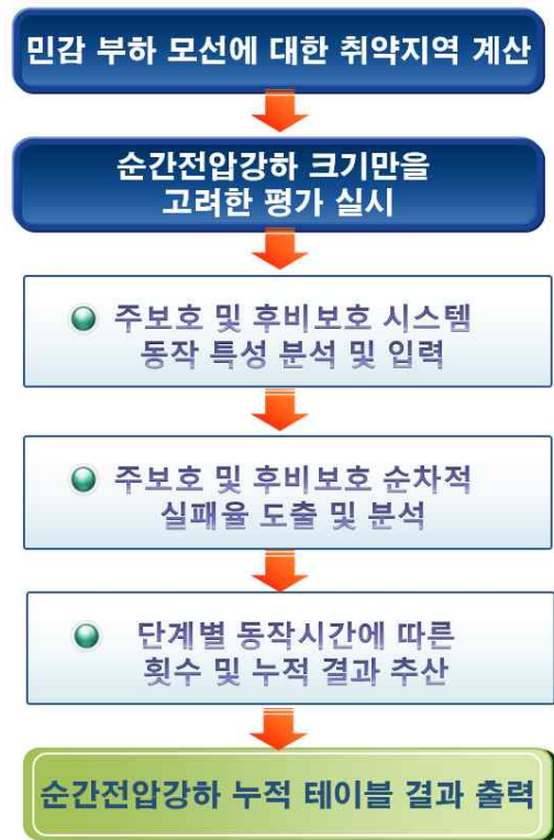
Fig. 5. Procedures of voltage sag assessment considering duration
