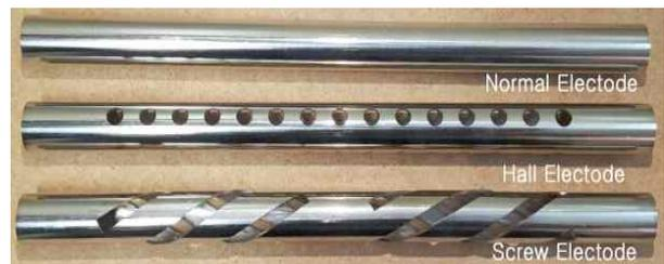
Fig. 3. The Photographs of each inner Electrode (Normal, Hall, Screw)
