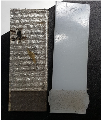
Fig. 6 Tensile test results of no-patterning
