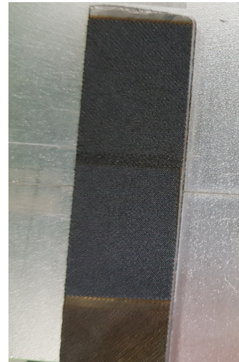
Fig. 7 Specimen of 3D printed metal plate with micro patterns on surface
