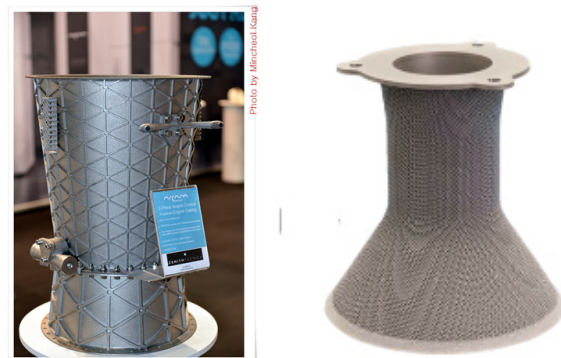
Fig. 7 Aerospace parts(up: F-15 part made by DED process, down: combustor made by PBF process)
