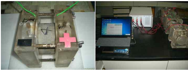
Figure 4. Arrangement for test to resist chloride ion penetration
