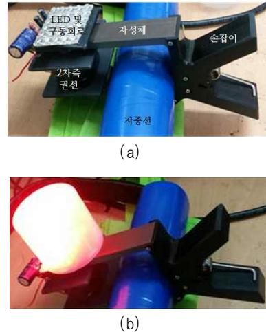
Fig. 11. (a) 60Hz 2W Wireless receiver prototype and (b) LED light operating.
