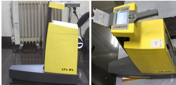
Fig. 7 Retroreflectivity Measurement
