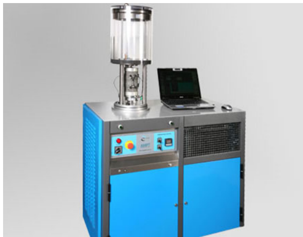
Fig. 6 Asphalt Mixture Performance Test (AMPT)
