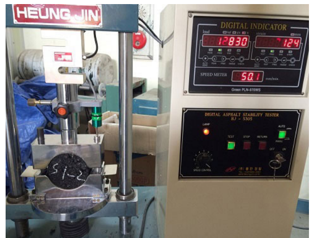
Fig. 1 Measurement of Marshall Stability
