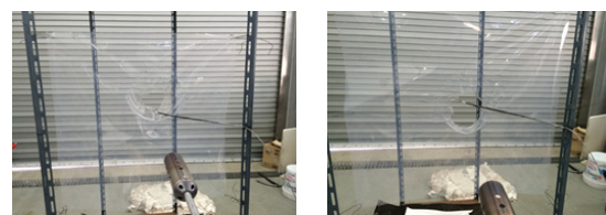
(a) 200mm (b) 300mm <Fig. 5> Fire characteristics (ETFE)
