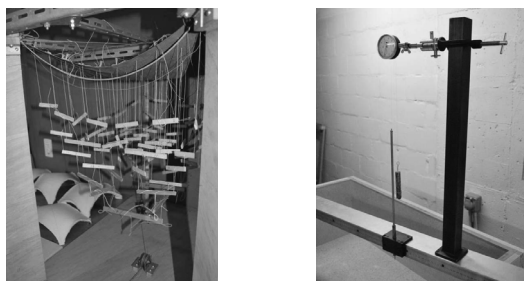
(a) Mechanical form-finding rig (b) Measurement jig
