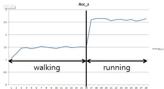
Fig. 1 z-axis sensor waveform of walking and running
