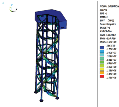
Fig. 10 Stress distribution of observation antenna (Normal condition)
