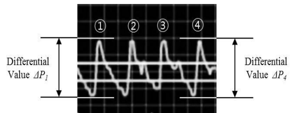
Fig. 5. Differential Values \Delta P_1 and \Delta P_4 from Arterial Pulse Waveform ① and ④
