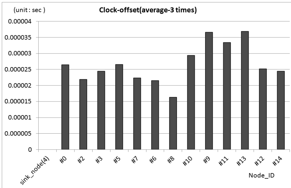
Fig. 4. Clock offset measurement(Synchronization error) for each node referenced to Sink node.
