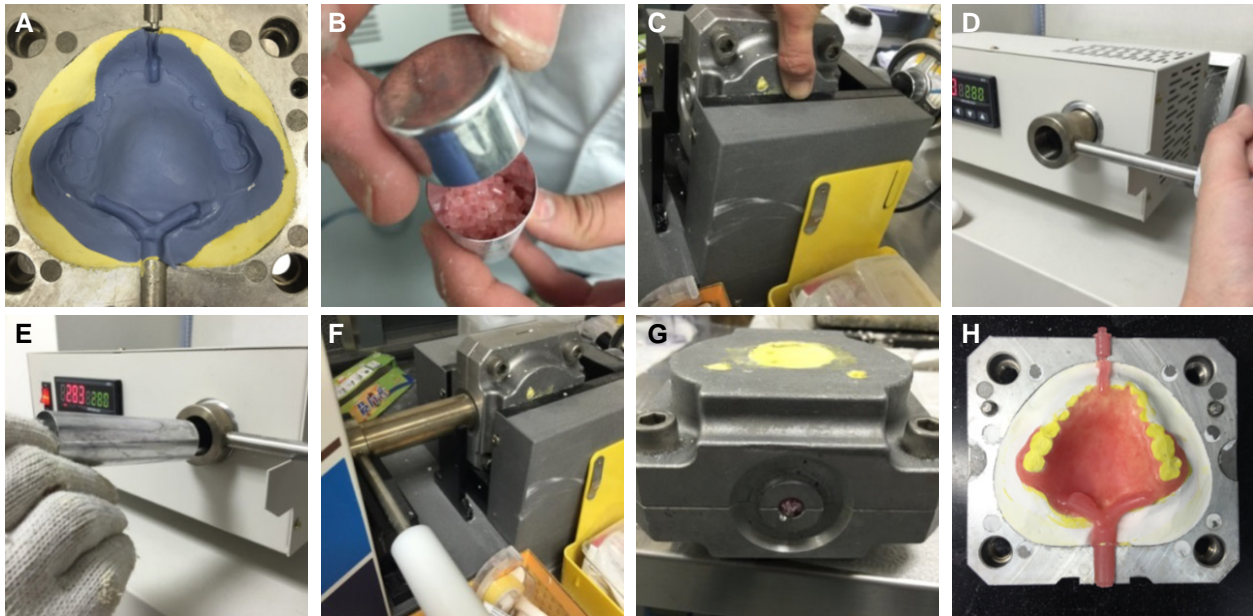
Fig. 4. Flasking & packing process. (A) Putty investment, (B) Thermoplastic pellets, (C) Special flask for injection molding technique, (D, E) Pellets in a cartridge plasticized in an electric furnace, (F) Cartridge placed on the inlet of the flask and compressed, (G) Cooling, (H) Deflasking.
