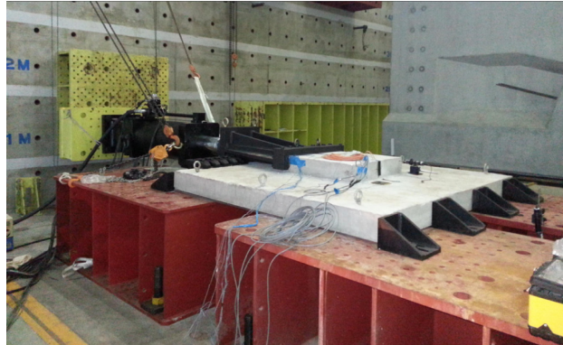
Fig. 8. Test set-up for shear key [14].
