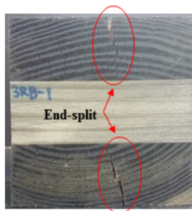
Fig. 4. End-split occurred in the outer lamina during the drying process of the boiling delamination test.
