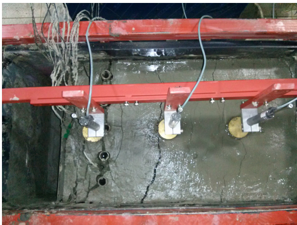
(a) Stabilizing pile : 5EA ( D_1/D_2 = 0.66 )
