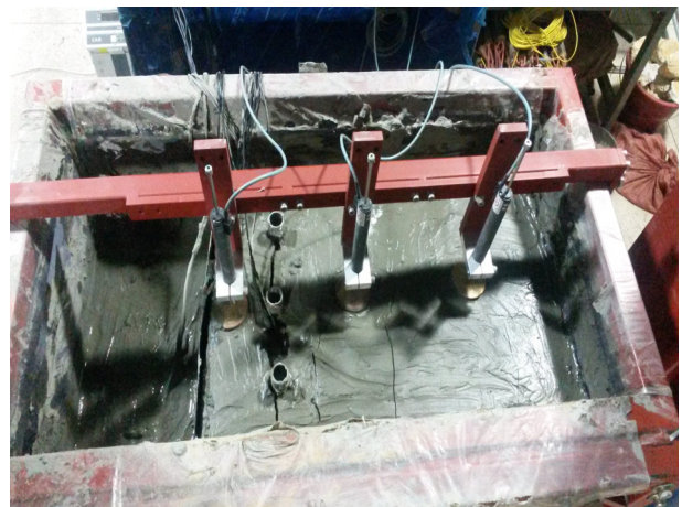
(b) Stabilizing pile : 3EA ( D_1/D_2 = 0.76 )
