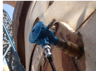
Fig. 8. Measurement system installed in the straight pipe of pneumatic transport of raw materials
