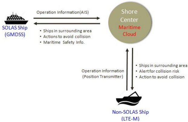
Fig. 1. Scenario of Ship Collision Prevention Support System (An, 2015).
