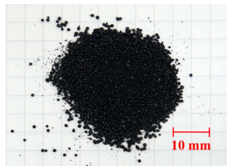
Fig. 1. Particle shape of rapid-cooled, electric arc furnace oxidizing slag (REOS).
