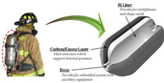
Fig. 1 Structural concept of Type3 cylinder
