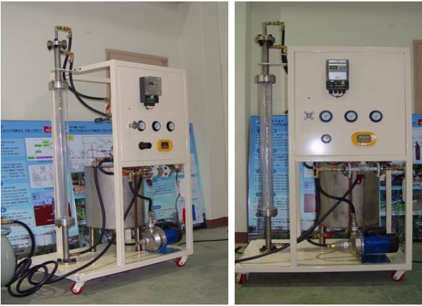
Fig. 2 The equipment of oxidizer feed flow characteristics test of the GPR-WAO
