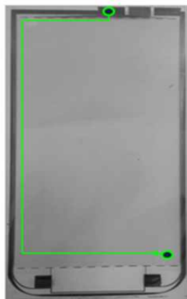
Fig. 10. 5.01 inch TSP sample. of CuN x -Cu-CuN x .
