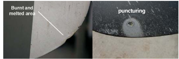
Fig. 6 Lightning strike on metal and composite blade [8]
