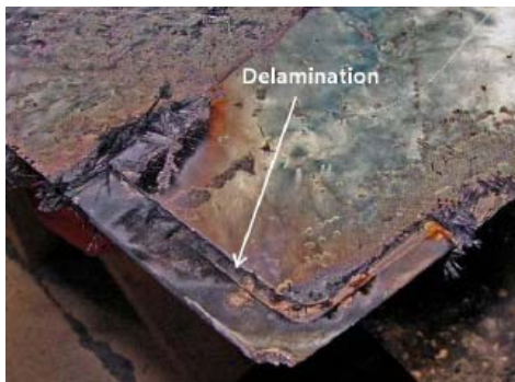
Fig. 3 Effect of lightning strike on conductive composite [6]
