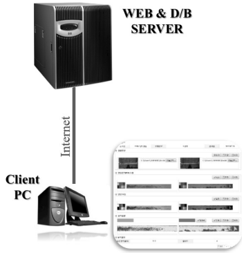
Photo 2 Architecture of computer-aided diagnosis system for Transmission Tower Steel Member
