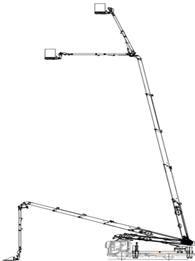
Fig. 1 Aerial work device with bend-linked boom
