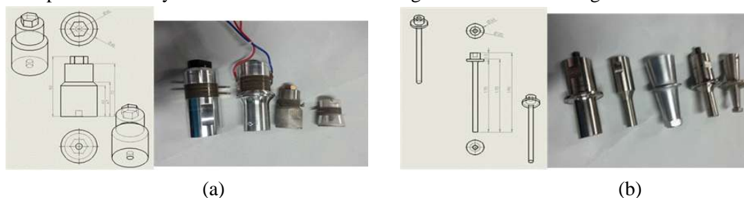
Figure 4. (a) Ultrasound Vibrator Design (b) Ultrasound Horn Design
