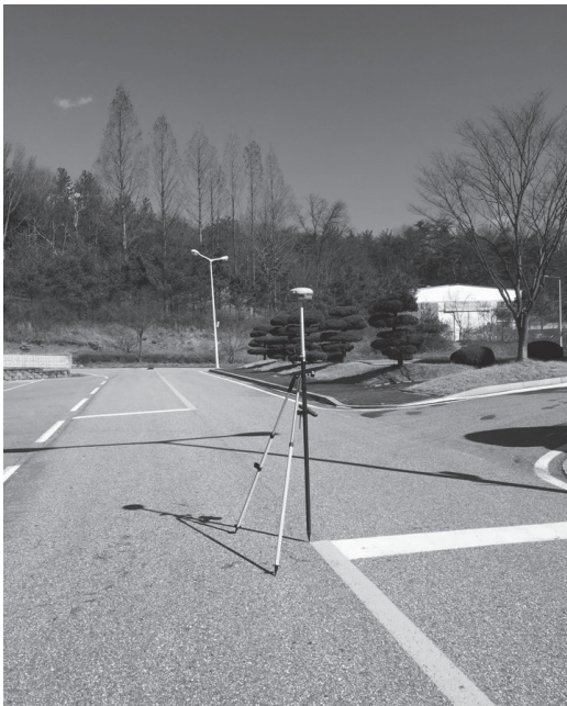
Fig. 3. GCP surveying with Network-RTK
