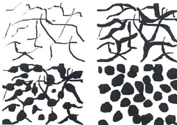
Figure 2-3-2. Time evolution in a sol-gel system of developing phase separation.
