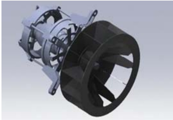
Fig. 3. Convection fan and motor
