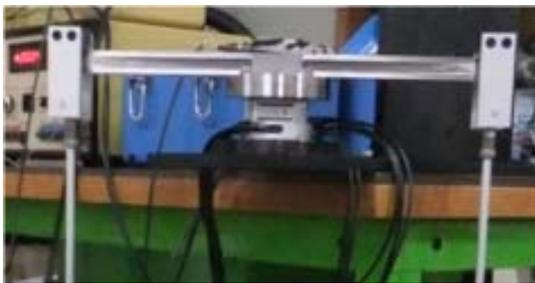
(b) Force  $F_z$  and Moment  $M_x$ ,  $M_y$ **Fig. 6** Experimental setup of 6-component force/moment generator developed
