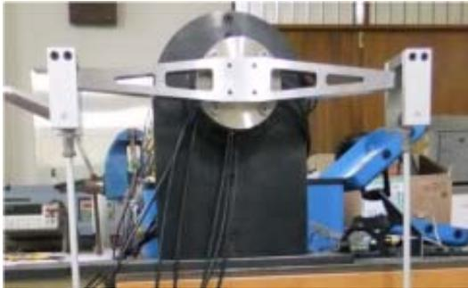
(a) Force  $F_x$ ,  $F_y$  and moment  $M_z$
