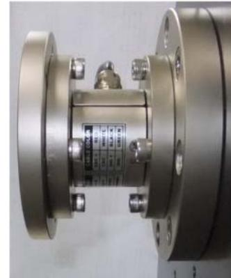
**Fig. 7** Moment test using a commercial torque cell
