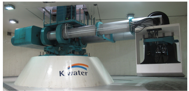
Fig. 1. 800g-ton geotechnical centrifuge
