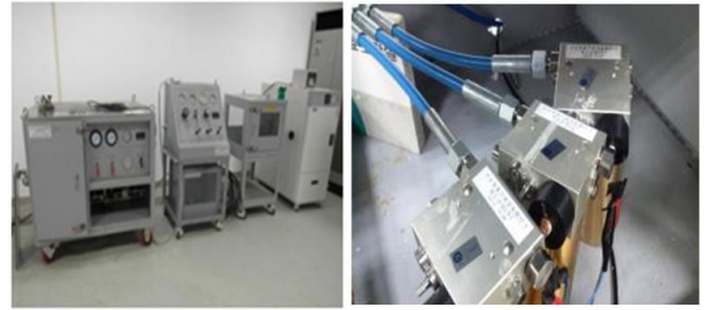
Fig. 10 Test equipment and installation status for cylinder valve
