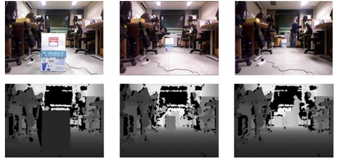
Figure 8. Sample images to estimate regression function according to distance; left, middle and right images represent when 60 cm, 400 cm and 700 cm, respectively.
