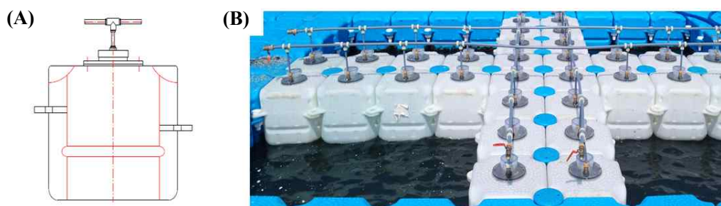
Figure 4. Shape of MPBR-HDPE. (A) schematic diagram; (B) MPBR-HDPE in local marine culture.
