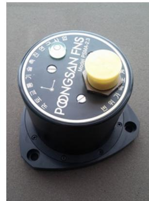
Fig. 1 Developed three-axes force-feedback accelerometer
