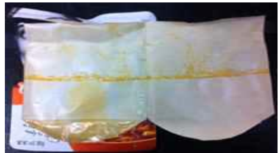
Fig. 6. Temperature measurement using a thermo-sensitive tape (left), and deformation of the package (right) used for a spicy chicken stew with black bean sample after microwave heating at 700 W for 2 min.
