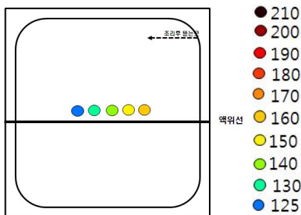
Fig. 6. Temperature measurement using a thermo-sensitive tape (left), and deformation of the package (right) used for a spicy chicken stew with black bean sample after microwave heating at 700 W for 2 min.
