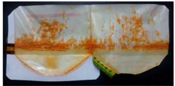
Fig. 5. Temperature measurement using a thermo-sensitive tape (left), and deformation of the package (right) used for a spicy chicken sauce sample after microwave heating at 700 W for 2 min.
