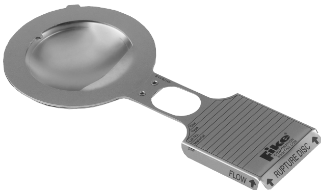
Fig. 5. The reverse buckling type rupture disc (the dome points towards the fluid under pressure) is similar to the one installed on the incident storage tank. Proper flow direction of pressure release is marked on the nameplate. (Photo courtesy of Fike Corporation.)
